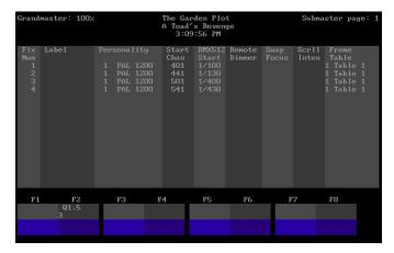
To display the Fixture List on the Playback display, press [Fixture List] on an ML console, or follow these steps.
