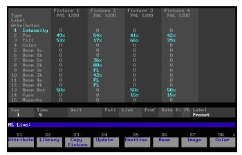
The [Expand] key functions in ML displays as it does in conventional displays, allowing you to see five additional fixtures on the Playback display. It is toggled on by the Expand button in the same manner that the Live Expand Display is for Channels.
