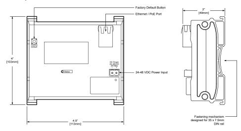
To factory default the device, press and hold this button for a 5 full seconds. This will perform a full factory default.
