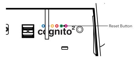
Insert a USB drive loaded with Cognito<sup>2</sup> firmware into one of the available USB ports, and then shut down the Cognito<sup>2</sup>. Using a plastic-coated paperclip or similar **non-metallic** small tool, insert it through the hole in the panel. Press and hold down the button while booting up the console with the power button. Keep the reset button pushed until the Cognito shows you the "**System Recsue**" screen.
