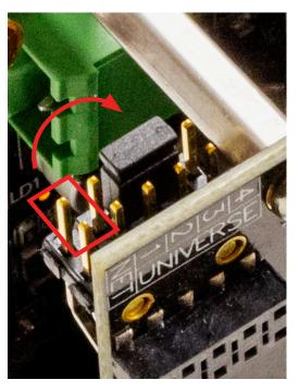
Once the jumper is placed in this position, the UNO **will be factory defaulted immediately.** There is no need to wait 5 seconds. Place the black jumper back in the "**NET**" position (or whatever position it was originally in, if hard-patching Universes), and put the UNO back in the enclosure.
