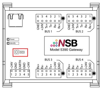
To factory default the device, press and hold this button for a 5 full seconds. This will perform a full factory default.
