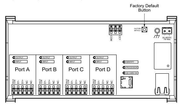
To factory default the 6824, press and hold the button for 5 seconds. This will perform a full factory default.
