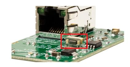
To factory default the device, press and hold this button for a **5 full seconds. This will perform a full factory default.** Use a **non-metallic** small tool to avoid shorting out any electrical contacts or transmitting an electrostatic discharge to the board.
