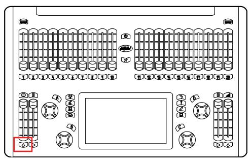
Continue holding the shift key until the Cognito<sup>2</sup> is finished booting. A new, blank show file should be loaded, without any passwords enabled.
