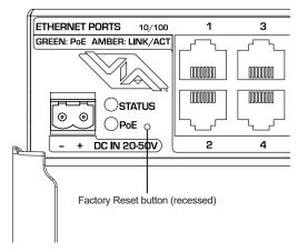
Using a plastic-coated paperclip or similar **non-metallic** small tool, insert it through the hole in the panel. Press and hold down the button for a **full 5 seconds. This will perform a full factory default.**
