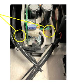
Removing the input power supply
