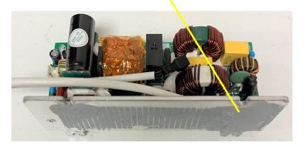
Removing the Output power supply
