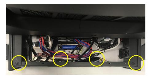
Remove 4X Philips head screws on front and rear top covers
