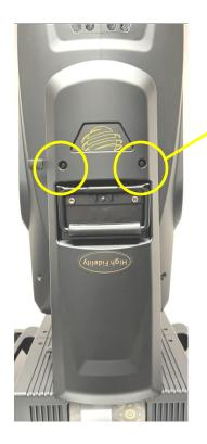
Remove 2x Phillips head screws on each yoke arm cover
