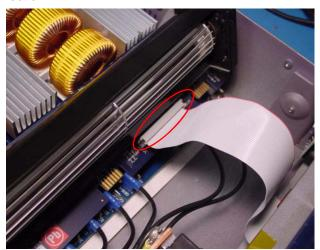
Step 9: Place new control card and fan assembly in position. Evenly push down with hands to make connection. After the card is secure, replace the two screws that hold the control card in place. If you do not have an assembled control card and fan assembly please see Additional Information #2.
