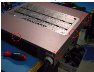
Step 2: After all (7) screws are out, remove the lid by sliding it back towards the power cable, then lifting it off and out of your way.
