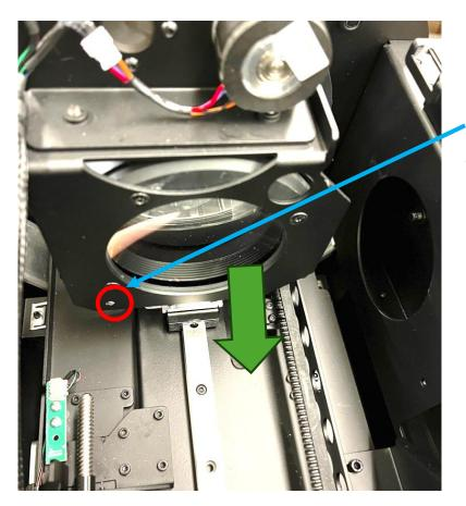
4. Carefully pull the zoom lens assembly toward the rear of the unit to remove it from the zoom rail mount.
