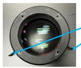
7. Ensure that the lens mounting bracket is at the bottom before continuing
