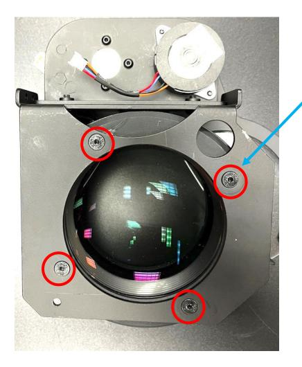
5. Remove the 4 countersunk screws using a 2.5mm hex tool
