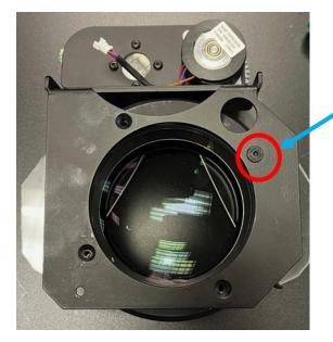
9. Use the provided screws to start threading all 4 before tightening. Tighten all screws using a 2.5mm hex tool.
