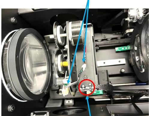
1. Disconnect the wires from the motor and sensor
