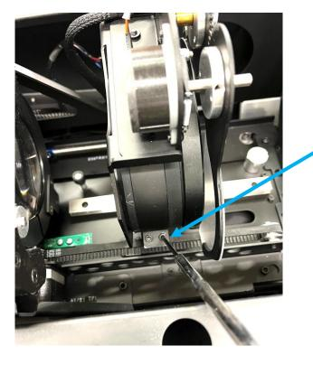
3. Remove 4 screws using a 2.5mm hex tool. There are 2 screws on each side of the zoom lens assembly
