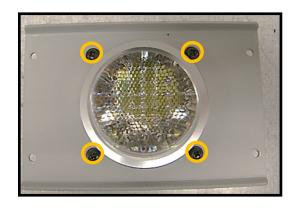
Remove 4X Philips head mounting screws
