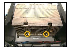
Remove 2X Philips head screws per side to remove LED Heatsink Remove 4X smaller screws
