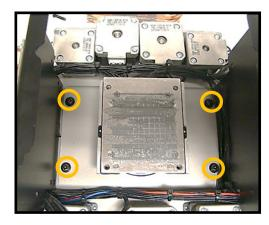
Remove 4X Philips head screws to remove LED mount
