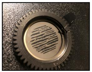
Once the holder is removed, unclip the metal tension spring that is holding the gobo in place Be sure the black or coated side of the gobo is facing <u>away</u> from the LED Light Engine
