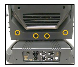
Remove 2X inner yoke cover screws and 4X outer yoke cover screws
