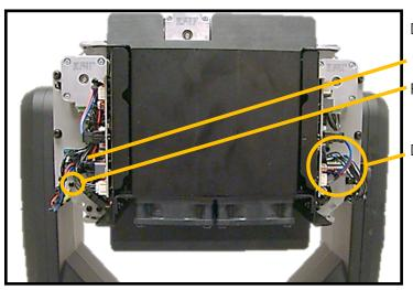
Disconnect first power and data wires
