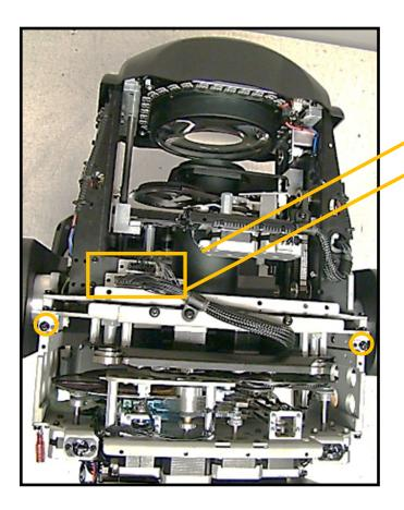
With the covers removed, lock the head of the fixture horizontally Push the zoom lens assembly forward Disconnect 2 Sub harness connectors Remove 2X Philips head screws Carefully pull out module
