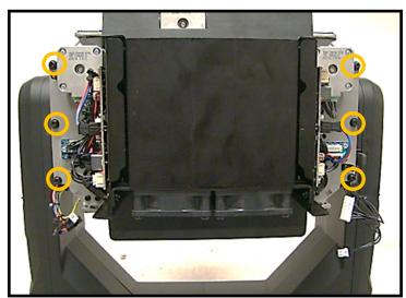
Remove 3X Philips head screws on each side while supporting the module
