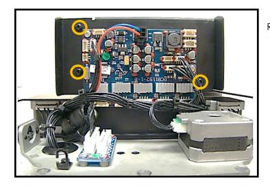
Remove 3X Philips head screws per side to remove fan plate housing
