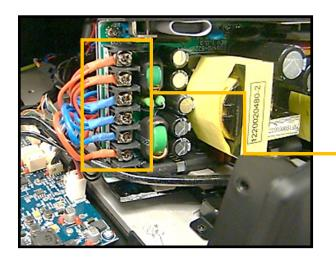
Loosen 6X silver Philips screws to disconnect output wiring Red Double Wire: 28VDC Positive (each) Red Single Wire: 52VDC Positive (each) Blue Double Wire: 28VDC Negative (each) Blue Single Wire: 52VDC Negative (each)
