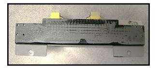
Remove power supply Be sure to mind the heatsink compound on the bottom Add heatsink compound to new power supply **before** installing
