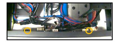
Remove 2X inner Phillips head screws on front and rear panels
