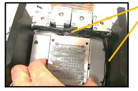
Slightly lift LED mount to disconnect LED harness Carefully remove LED, mind the wire harness while removing
