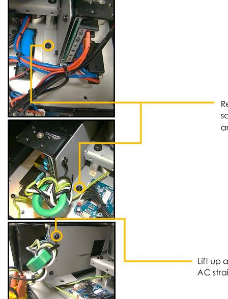
Remove 2X Phillips head mounting screws next to the display battery and next to the LED Control PCB
