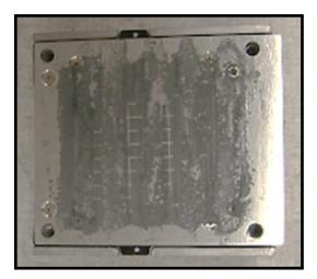
Apply heatsink compound to the new LED Light Engine before installing
