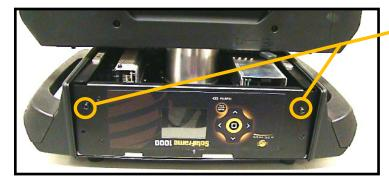
Remove 2X Philips head screws on the front and rear panels
