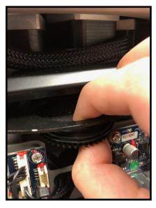
To remove both the static and rotating gobos from the wheel, removing the module is not required
