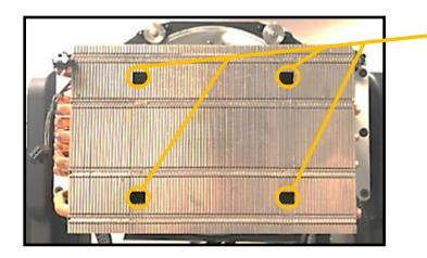
Remove 4X Philips head screws to remove LED heatsink
