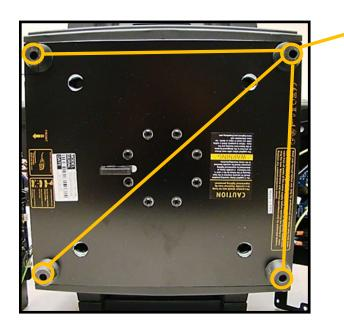
Remove 4X rubber feet using 3mm Hex tool
