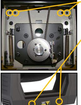
Remove 2X Philips screw heads
