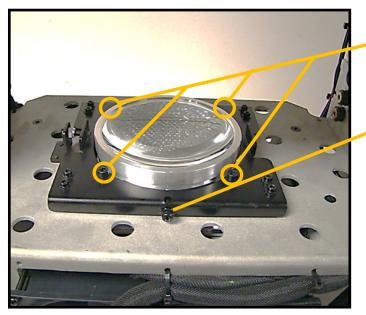
Remove 4X screws using 3mm Hex tool
