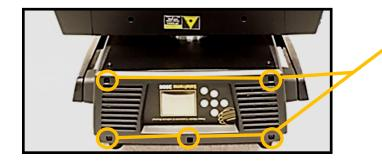
Remove 5X Philips head screws on the front and rear plastic covers
