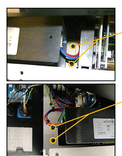
Remove 2X Philips head front mounting screws Using a magnetized Philips head is ideal Remove LED control PCB/LED distro PCB mount for more room if necessary
