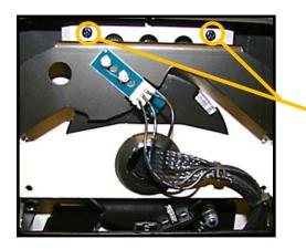
Remove 2X Philips screw heads Using a magnetized screwdriver would be ideal
