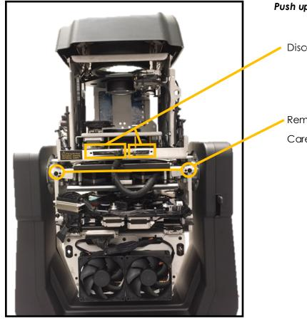
Push up focus lens to clear module or tilt head downwards
