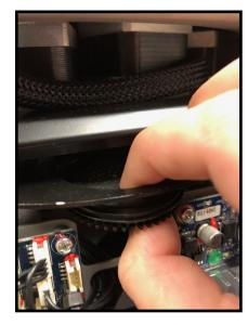
To remove both the static and rotating gobos from the wheel, removing the module is not required
