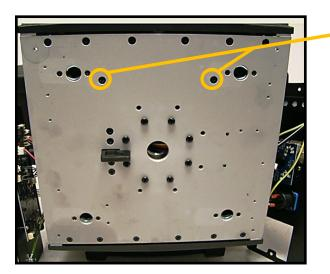
Remove 2X Philips head screws
