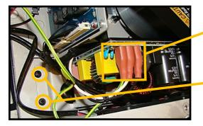
Disconnect input power connections
