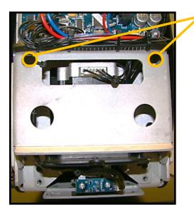
Remove 4X Philips screw heads through access holes
