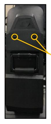
Loosen 2X Philips head screws on each arm cover to remove
