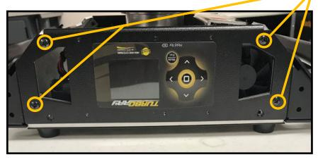
Remove 4X Philips head screws on front and rear panels
