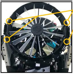
Loosen 4X Philips head screws to remove the primary diffusion
