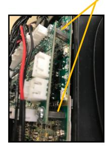
Removing the LED Driver PCB 2
