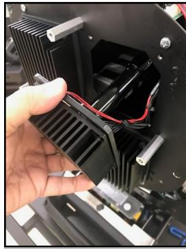
Remove the LED Light Engine one at a time and be sure to replace in the same position and orientation
