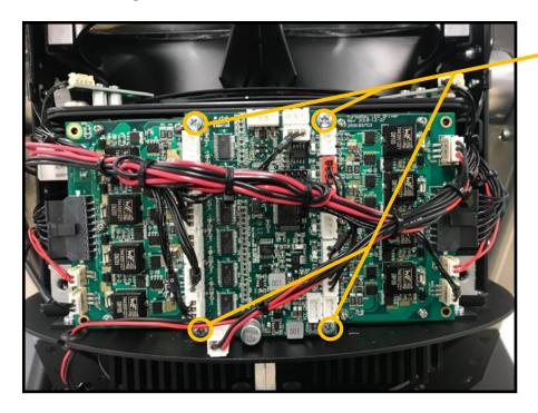
Disconnect wires going into the PCB
