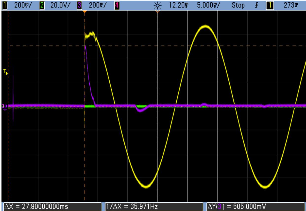
The yellow trace is the mains waveform – power has just been turned on. The purple trace is current (20A per division). The current peak is 50.5A, but as you can see for a very short period – about 2.5 milliseconds (0.0025 seconds)
