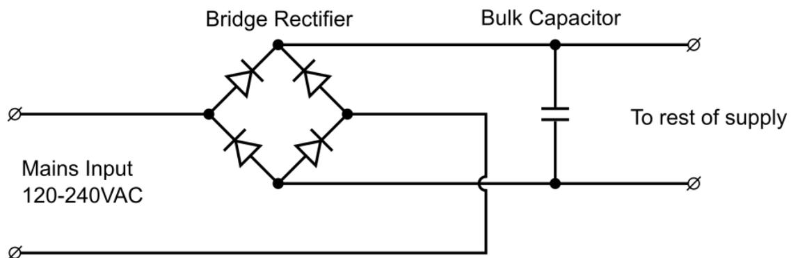
If you think of electricity like water, the bulk capacitor you can think of like an empty tank. When the circuit first has power applied, water flows into the tank very quickly; once the tank fills up, there's no space for more water, so no water flows in. That initial fast flow is exactly what our inrush current is – current rushing in to fill up the bulk capacitor.
