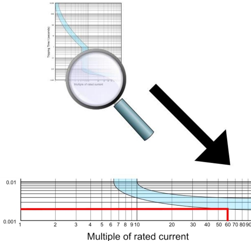
By following across the 0.002 second line, we see this breaker can hold 60 times its rated current at this timespan.
