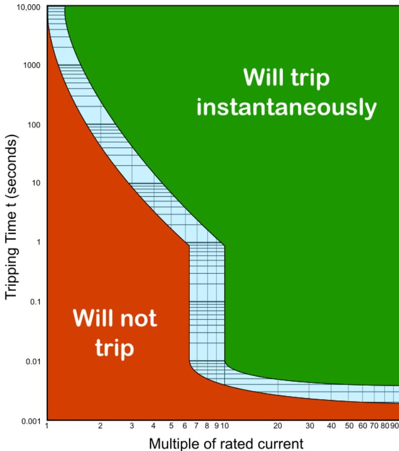
This makes it easier to understand. If a particular point is in the red, left-hand region, the breaker will not trip when subjected to those conditions. If a point is in the green, right-hand region, it is guaranteed the breaker will trip.
